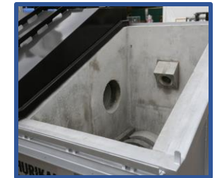
Inside view of AIS1250 Cyclone main chamber
